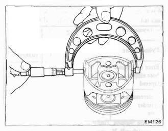
Fig. EM-43 Measuring the piston diameter
