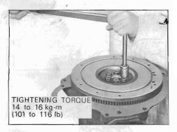
Fig. EM-80 Flywheel installation
