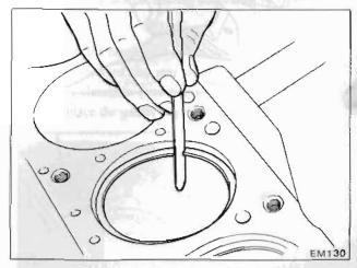
Fig. EM-48 Ring gap measurement
