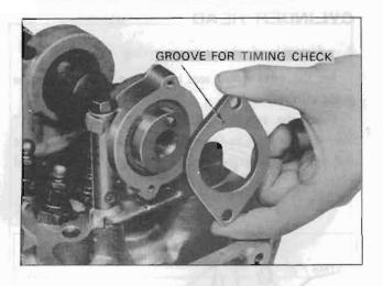
Fig. EM-72 Camshaft locating plate installation
