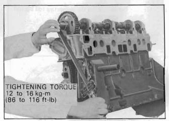
Fig. EM-89 Fuel pump cam installation
