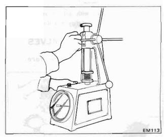
Fig. EM-31 Valve spring test
