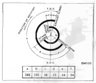
Fig. EM-38 Valve timing diagram
