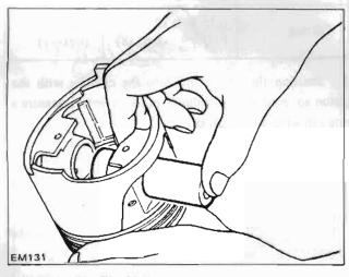
Fig. EM-49 Piston pin fitting
