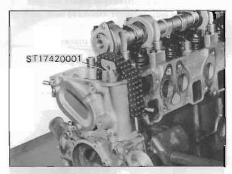
Fig. EM-12 Camshaft drive sprocket removal
