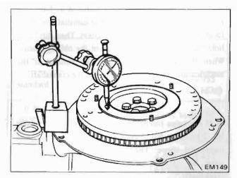
Fig. EM-66 Checking flywheel runout
