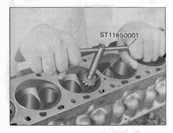
Fig. EM-35 Valve seat correction
