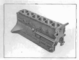
Fig. EM-2 Cylinder block
