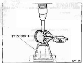
Fig. EM-73 Piston pin installation
