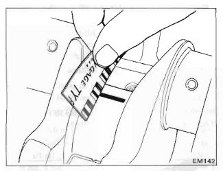
Fig. EM-59 Bearing clearance check
