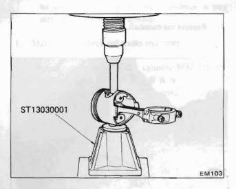
Fig. EM-21 Piston pin removal
