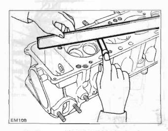
Fig. EM-27 Checking the cylinder head surface
