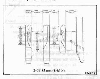
Fig. EM-53 Crankshaft dimensions
