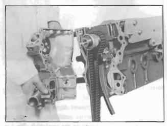
Fig. EM-14 Engine front cover removal
