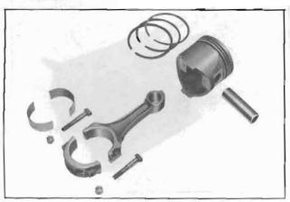
Fig. EM-4 Piston and connecting rod
