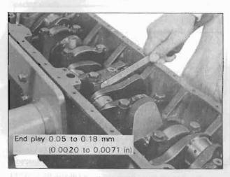
Fig. EM-55 Crankshaft end play check
