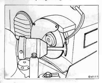
Fig. EM-29 Regrinding valve face
