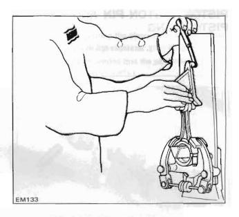
Fig. EM-51 Connecting rod alignment
