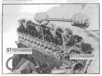
Fig. EM-13 Cylinder head removal
