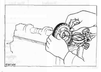
Fig. EM-62 Camshaft end play check
