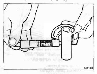
Fig. EM-50 Measuring piston pin diameter
