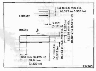
Fig. EM-32 Service valve guide
