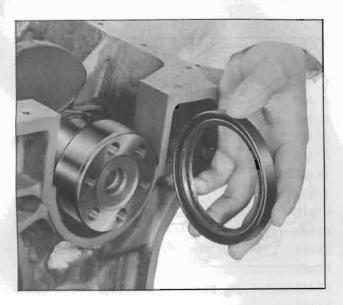
Fig. EM-18 Rear oil seal removal
