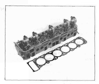
Fig. EM-5 Cylinder head
