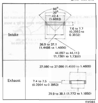
Fig. EM-36 Standard valve seat insert
