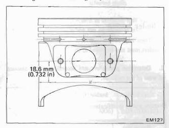
Fig. EM-44 Measuring point of the piston
