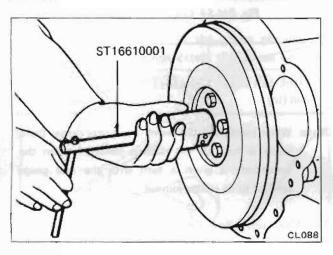
Fig. EM-56 Pulling out pilot bushing
