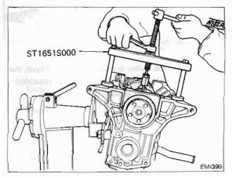
Fig. EM-17 Rear main bearing cap removal
