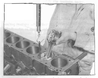
Fig. EM-45 Piston to cylinder clearance check
