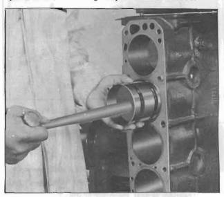
Fig. EM-81 Piston-rod assembly intallation
