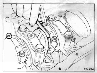
Fig. EM-77 Camshaft end play check
