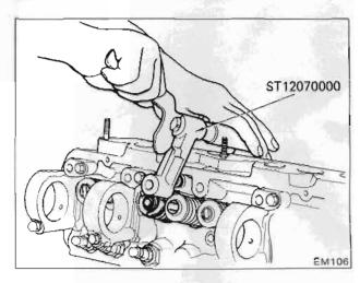
Fig. EM-24 Valve removal
