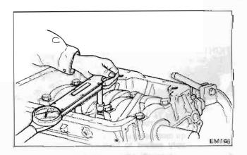
Fig. EM-82 connecting rod cap installation
