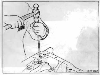
Fig. EM-78 Side oil seal installation
