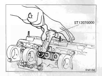
Fig. EM-71 Valve installation
