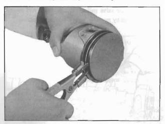
Fig. EM-20 Piston ring removal
