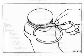
Fig. EM-47 Side clearance measurement
