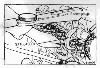
Fig. EM-95 Adjusting valve clearance
