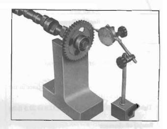
Fig. EM-61 Camshaft sprocket run-out check
