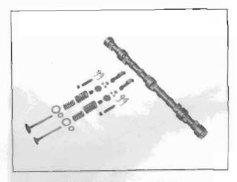
Fig. EM-25 Valve components
