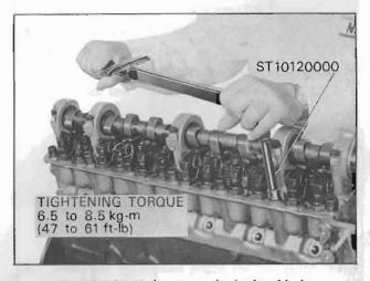
Fig. EM-86 Tightening cylinder head bolts
