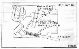
Fig. EM-33 Valve guide installation
