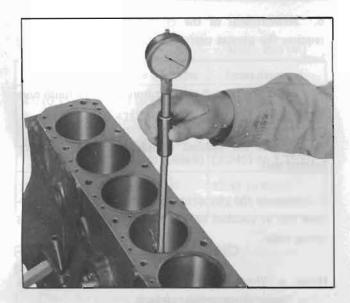
Fig. EM-41 Measuring the cylinder bore
