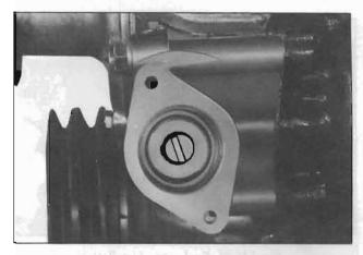
Fig. EM-92 Setting the distributor driving spindle
