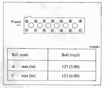
Fig. EM-84 Cylinder head bolts
