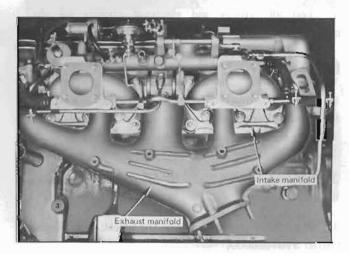
Fig. EM-9 Intake and exhaust manifolds
