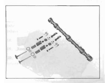
Fig. EM-7 Valve mechanism
