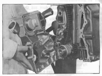
Fig. EM-90 Front cover installation
