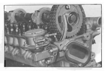
Fig. EM-94 Fuel pump installation
