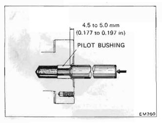
Fig. EM-57 Press-fitting new pilot bushing
