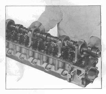
Fig. EM-23 Camshaft removal
