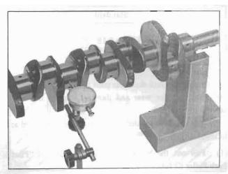
Fig. EM-54 Crankshaft bend check
