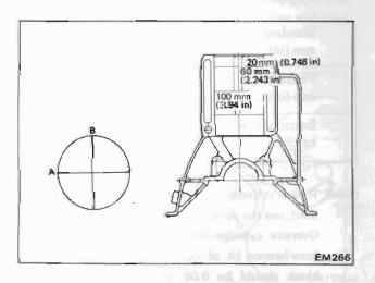
Fig. EM-42 Measuring points of cylinder bore
