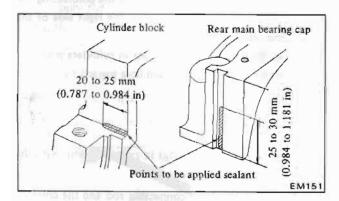
Fig. EM-69 Applying sealant (Main bearing cap and cylinder block)
