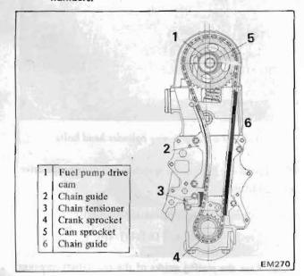
Fig. EM-88 Timing chain installation
