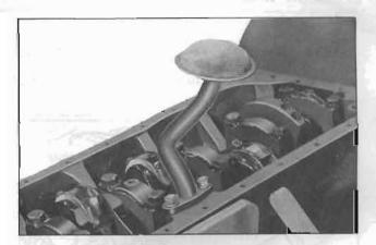
Fig. EM-93 Oil strainer installation
