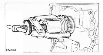
Fig. EM-15 Chain drive sprocket removal
