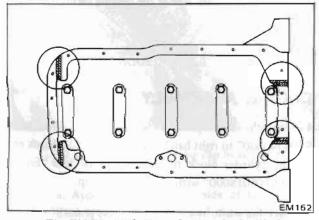
Fig. EM-70 Applying sealant (Cylinder block)
