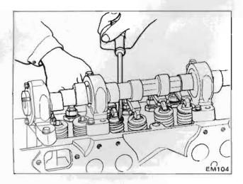
Fig. EM-22 Rocker arm removal
