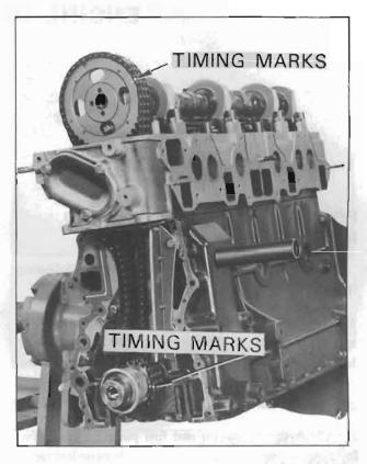
Fig. EM-8 Camshaft driving chain
