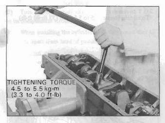
Fig. EM-76 Main bearing cap installation
