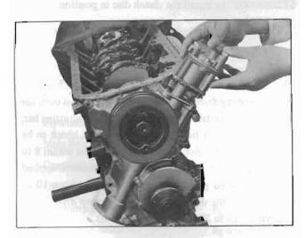
Fig. EM-91 Oil pump installation
