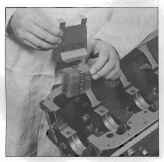
Fig. EM-19 Buffle plate and net removal
