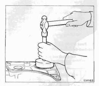
Fig. EM-79 Rear oil seal installation
