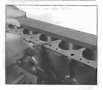
Fig. EM-40 Cylinder block surface check
